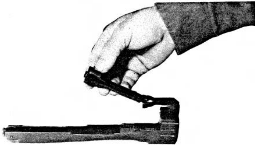
FIG. A-8. BOLT REMOVED FROM CARRIER BLOCK
