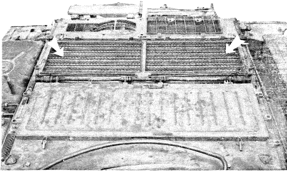
FIG. 1-7. ENGINE AND POWER TRAIN DECK LIDS
